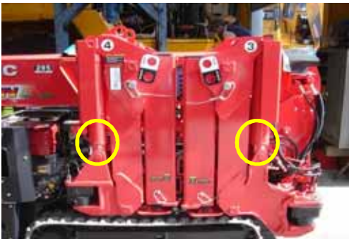
Load Cell is at the end of each outrigger cylinder. ( 4 Load Cells are on a crane )
