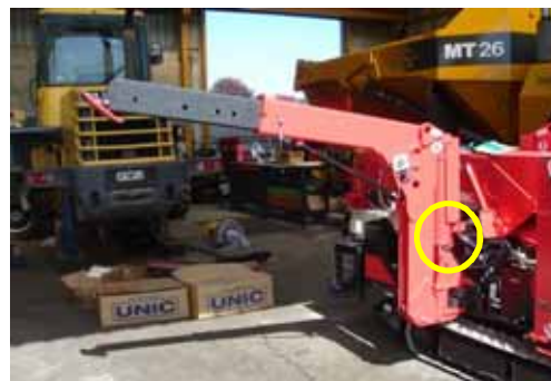
Load Cell is at the end of each outrigger cylinder. ( 4 Load Cells are on a crane )
